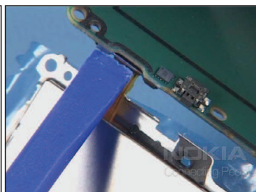
20. Carefully unlock the flex connector of the LCD MODULE.
