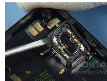
25. Carefully lever out the EARPIECE ASSEMBLY.
