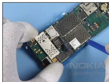
19. Unlock both metal clips of the UI SHIELD.
