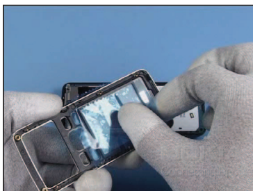
10. Protect the window from inner side.
