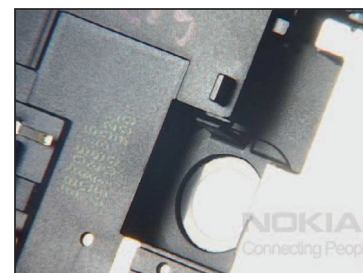
9. Secure all clips of the PLASTIC CHAMBER before going on.
