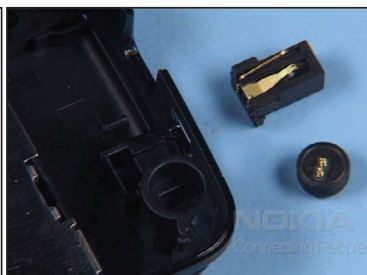
24. Remove the MICROPHONE and the DC JACK.
