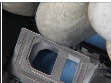
32. Turn the assembly and open the SIM lid.
